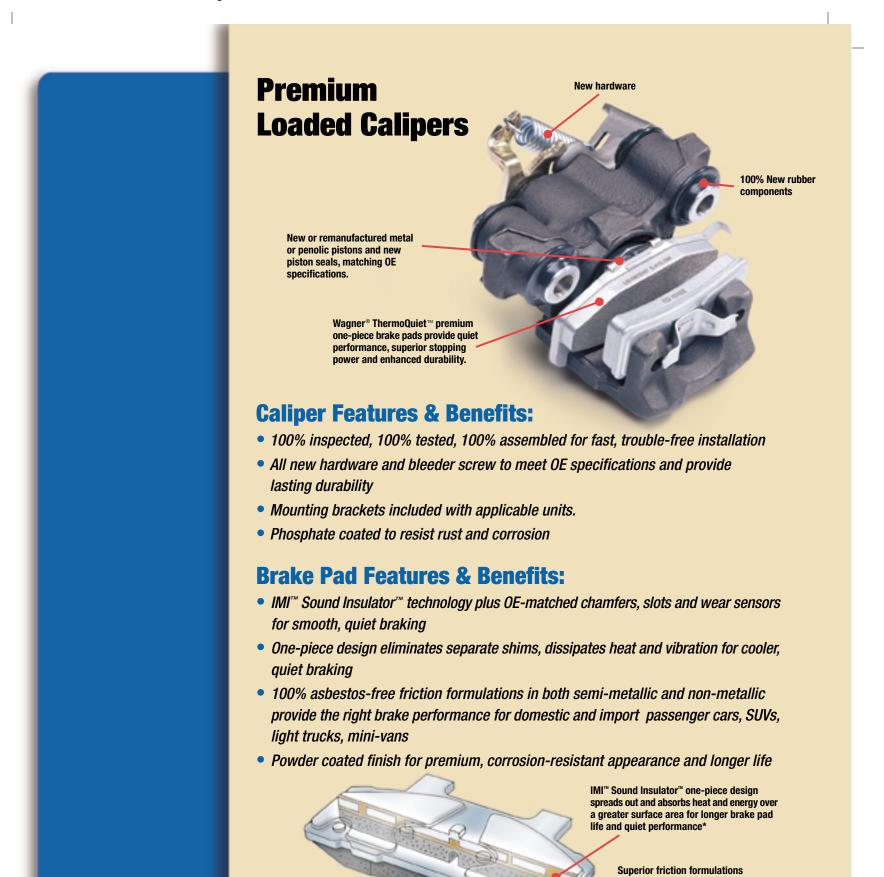
OE-matched chamfers, \_\_\_\_\_\_\_\_ slots and wear sensors engineered to pass 0.E. manufacturerdeveloped stopping test
