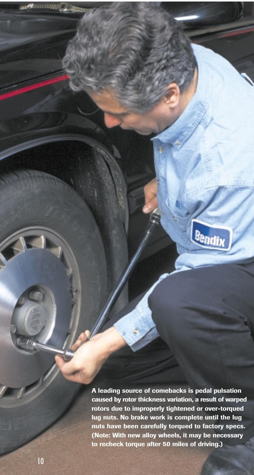
A leading source of comebacks is pedal pulsation caused by rotor thickness variation, a result of warped rotors due to improperly tightened or over-torqued lug nuts. No brake work is complete until the lug nuts have been carefully torqued to factory specs. (Note: With new alloy wheels, it may be necessary to recheck torque after 50 miles of driving.)
