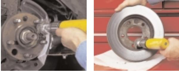
**Left:** Anytime a rotor has been removed, the job shouldn't be considered complete unless mating hub/rotor surfaces have been thoroughly cleaned. Otherwise, foreign material between the two items may cause runout, leading to a complaint of pedal pulsation.
