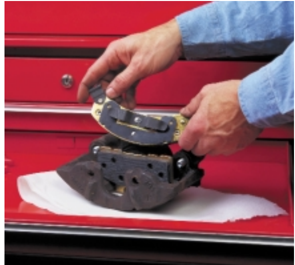
Some TSBs recommend a simple pad swap to get rid of brake noise.
