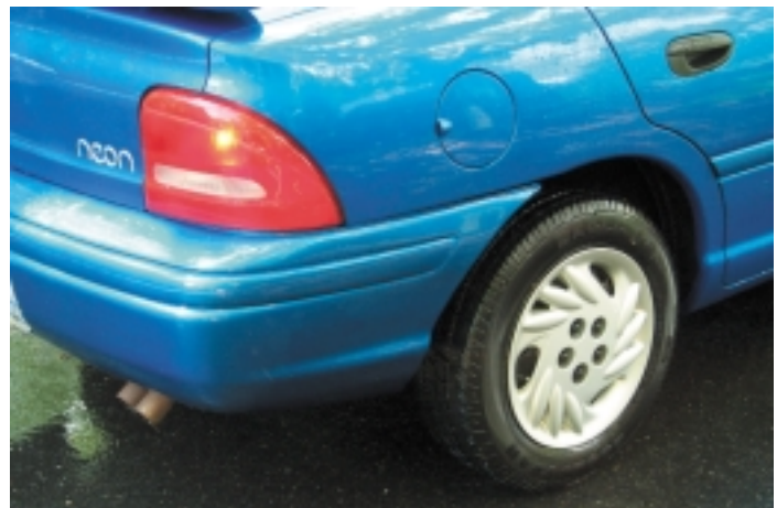
A Chrysler TSB says replacing the brake-shoe support plates is all you need to do to eliminate a rear-brake howl on some '95-97 Neons.
