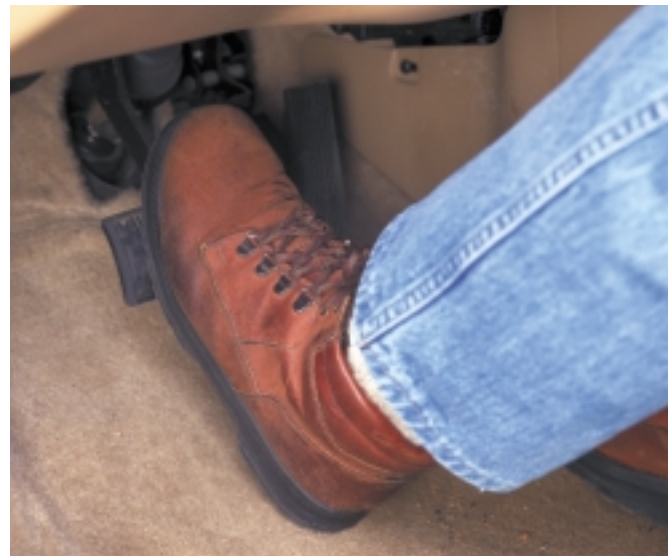
To be sure you've adjusted the brake-light switch properly, test the brake pedal while an assistant watches the brake lights.
