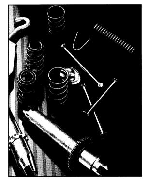
which can cause rust, leading to "freezing" of self-adjusting components which must be free to move in and out in order to work properly. Yet another potential problem area is the stretching of the self-adjusting cables, which can lead to mis-adjusted brakes.
