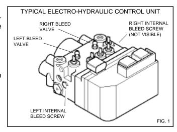
Clear all codes before performing the function test. Use a TECH 1 or jumper key (F121029). Run three tests to get fluid through the EHCU. After the function testing drive the vehicle and perform three to five ABS stops. The code(s) should then be clear. Check the Brake Bleeding Sequence Guide, an ABS manual or vehicle service manual for further information.
