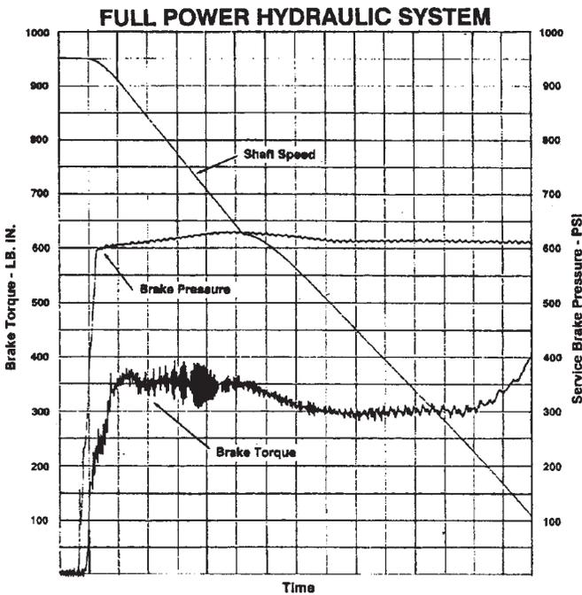
Figure 10 Time response - Full Power hydraulic
