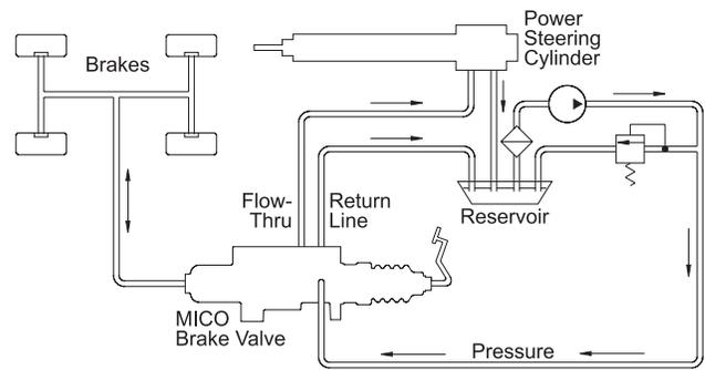
Figure 4 Open Center Power Brake System Typical Circuit
