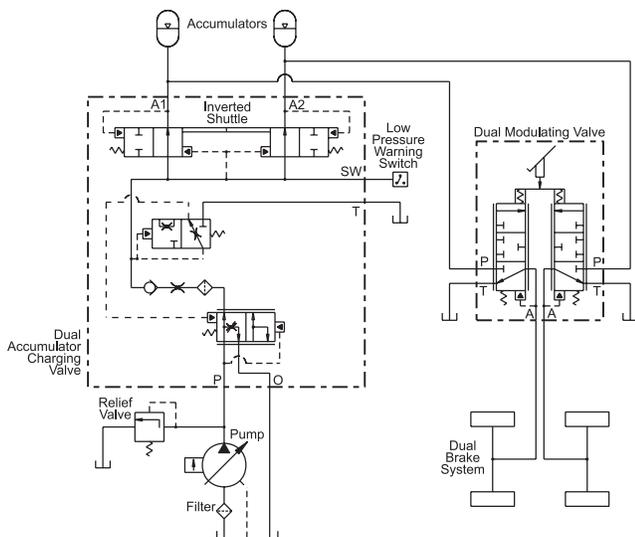
Figure 12 Dual Closed Center Brake Circuit in a Dedicated Open Center Hydraulic System
