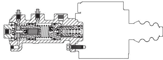
Figure 7 Two Fluid Tandem Master Cylinder
