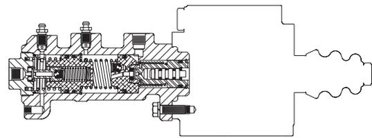
Figure 7 Two Fluid Tandem Master Cylinder
