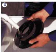
Never re-install a resurfaced rotor or drum before washing it with hot water and detergent. Rinse thoroughly and use paper towels to dry. This helps ensure that microscopic bits of metal left over from resurfacing won't embed themselves in the pads and shoes, altering their stopping performance.
