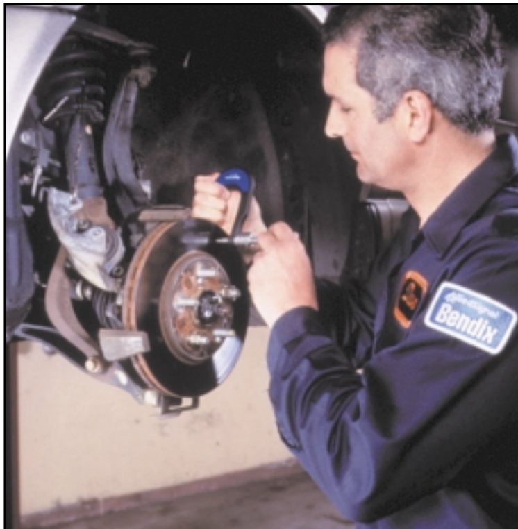
Measure rotor thickness at several points with a micrometer, and replace the rotor if any reading is at or below the "discard" specification. If all readings are above "discard" but thickness varies more than 0.005 inch, resurfacing is needed to prevent pulsation.
