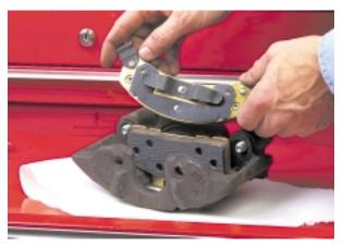
Surveys show that brake hardware is usually not replaced until it's so worn that it may lead to erratic brake operation. Installing fresh hardware at each friction replacement is part of a complete job that helps ensure proper brake performance and long service life.
